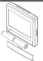
Press the touchscreen with your fingertip only, using a firm touch. Do not use a sharp object such as a pen or pencil. The touchscreen is a resistive touch and responds differently than touchscreens found in smart phones/devices.
